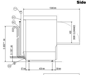
Without drain pump \*\*\*Plug only for Single Phase Machine
